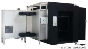
15°C to 75°C while measuring the electrical performance of photovoltaic modules. Nevertheless, the cetisPV-Therm2-M even allows for automated and quick measurements of a wider temperature range from 10°C to 80°C. Driven by a user-defined grid which describes the measurement series in detail for the whole temperature profile, temperature accuracy and temperature homogeneity exceed the demands of the IEC norm by far.
