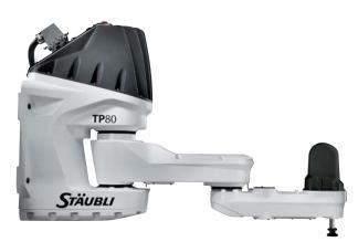
unlike rival delta robots. A simple base or wall mounting eliminates the need for a large, costly gantry, further enhancing the robot's cost effectiveness and ease of integration. Additional advantages include a slim forearm for moving into slotted machine openings as well as harness and user lines feed-through the Z-axis that are all internal. The TP80 fast
